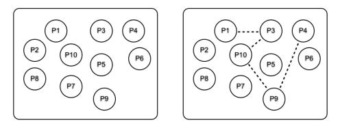
To create links, we call the primitive link(Pid), which creates a link between the calling process and Pid. So, if P1 calls link(P3), a link is created between P1 and P3.
