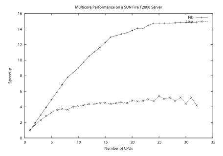
As we can see, CPU-bound computations with little message passing have linear speed-up, whereas lighter-weight computations with more message passing scale less well.
