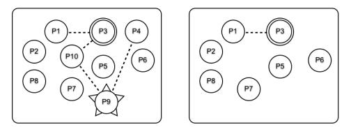
To achieve this, assume that P3 has evaluated process\_flag(trap\_exit, true) and become a system process (meaning that it can trap exit signals). This is shown with a double-circle border on the right side of the figure. After P9 crashed, the propagation of errors stopped at P3, so P1 and P3 did not die. This is shown on the right side of the figure.
