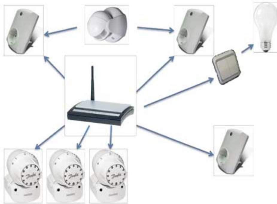
Z-Wave Network with single static controller
